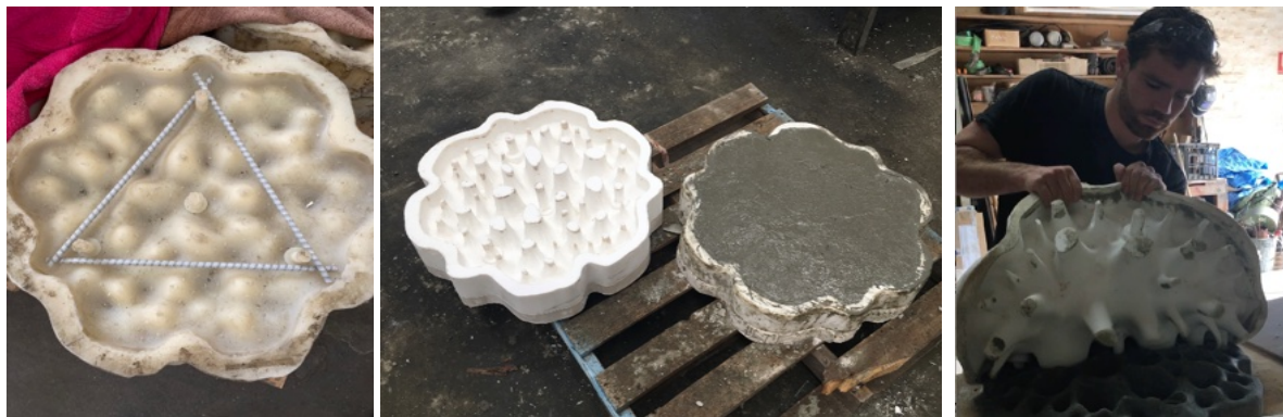
Figure 4: Images of panel fabrication. (Image credits: Alex Goad.)
