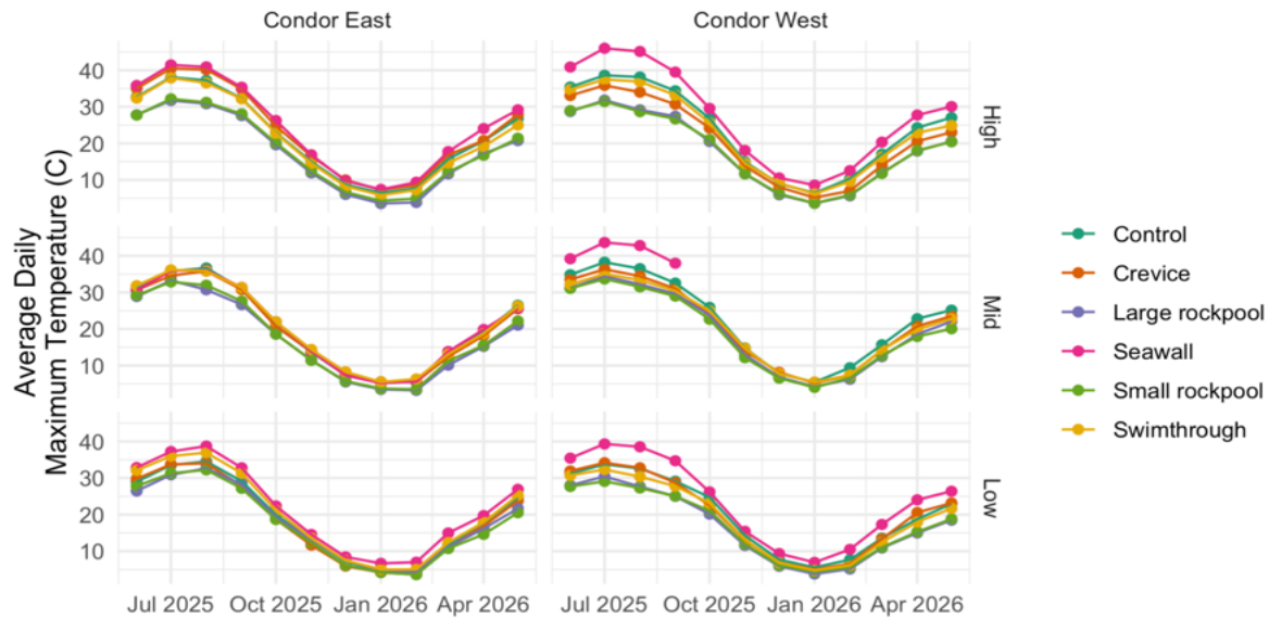
Figure 20: The average maximum daily temperature by month on different panel designs and the adjacent control seawall at Condor Street Urban Wild.
