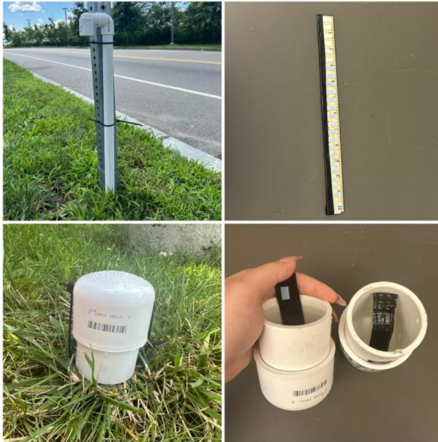
The flood measurement equipment. The photos on the left show the vertical (top) and horizontal (bottom) indicators deployed at a site. The photos on the right show the cobalt chloride paper in each indicator.
