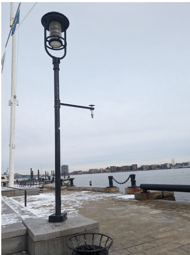
The Hohonu overland flood monitoring station at Long Wharf in Downtown Boston
