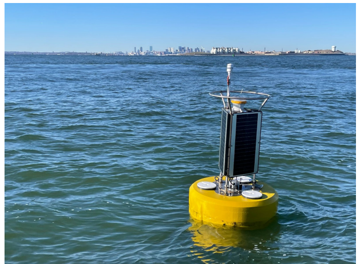
Wave Buoy at the entrance to Boston Harbor.
